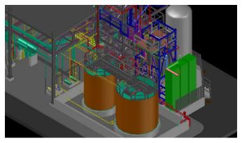
A 3D model created of the cryogenic plant created in CADWorx Plant Professional.
